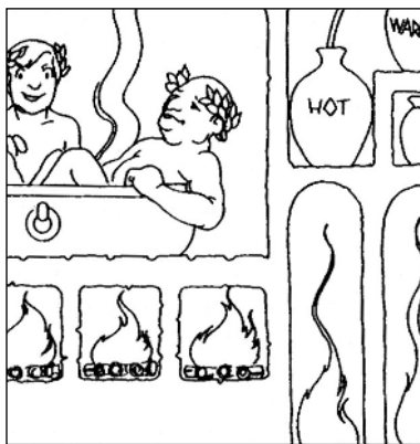
The Romans used a combination of convection and radiant heat in their ancient baths. The baths at Caracalla used technology like this.
